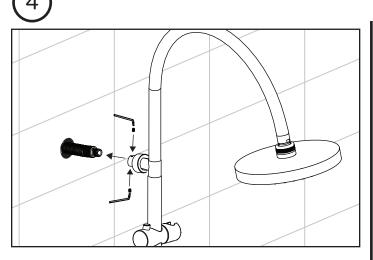
Attach assembled shower to inlet nipple (8) and secure set screws (4) with allen wrench (24) provided.
