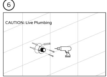
Drill wall mount (17), place it on marked location and mark holes for drilling. Set wall anchors (16) in place. Place the wall mount (17) on marked location for easy, steady, installation. Drill mounting screws (18) into place.
