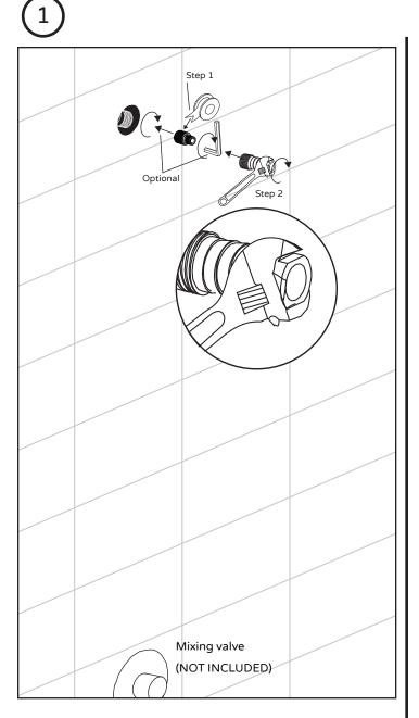
[Step 1] Apply a generous amount of PTFE (plumber's) tape to end of end of nipple.
