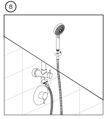
Attach swivel joint (22) to shower pipe (11). Insert washer (26) into the hex end of the handshower hose (15). Attach hose (15) to swivel joint (22) on the diverter body (19).
