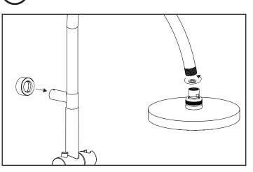
Slide escutcheon (6), insert washer (26), and screw showerhead (1) to shower arm (2) and secure.
