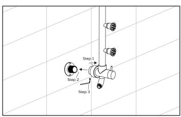
Step 1: Slide escutcheon (6) back in order to place set screw (4) later on.
